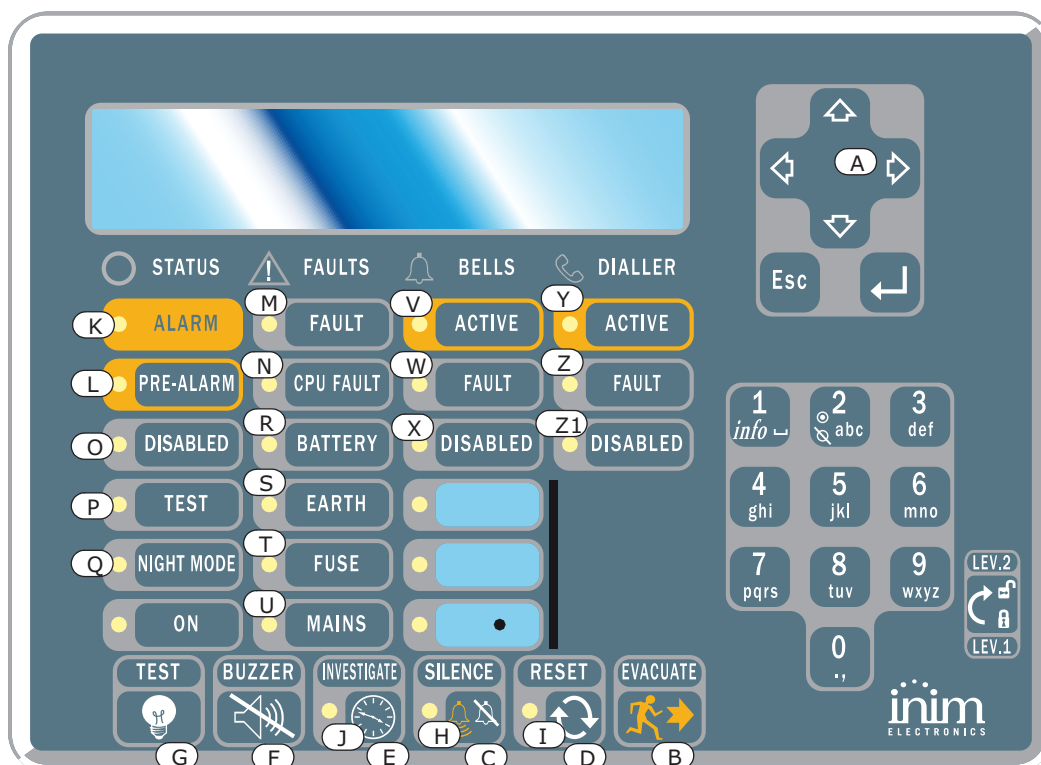
Figure 7 - Front view of the Repeater panel
