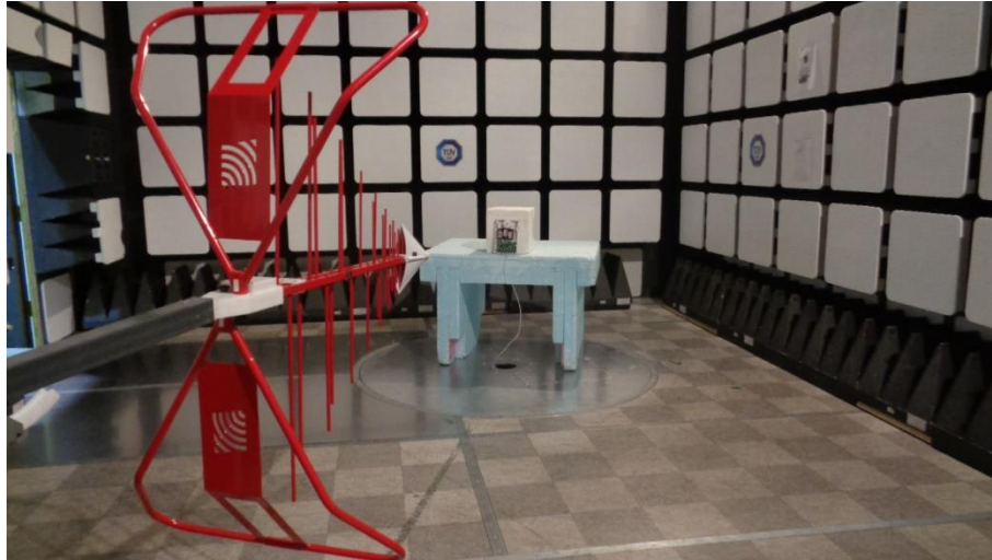
Photo 13 – Test Setup – Receiver Blocking – Inside the Chamber
