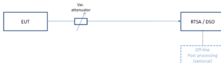
Figure 2: EUT – Setup Diagram – DCT Conducted Measurements
