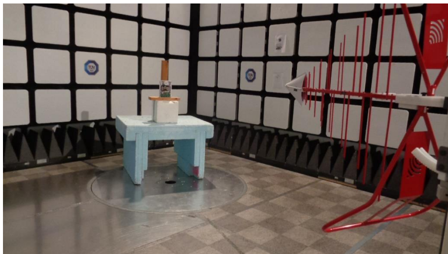
Photo 12: Setup – Tx Unwanted Emissions – SR250 – 30MHz to 1GHz – Vertical Polarization
