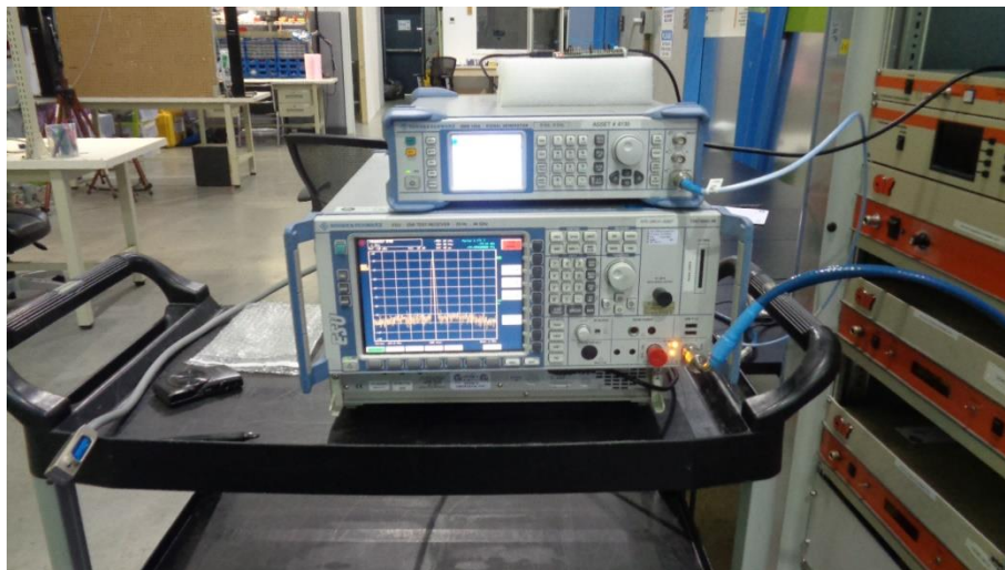
Photo 14 – Test Setup – Receiver Blocking – Outside the Chamber
