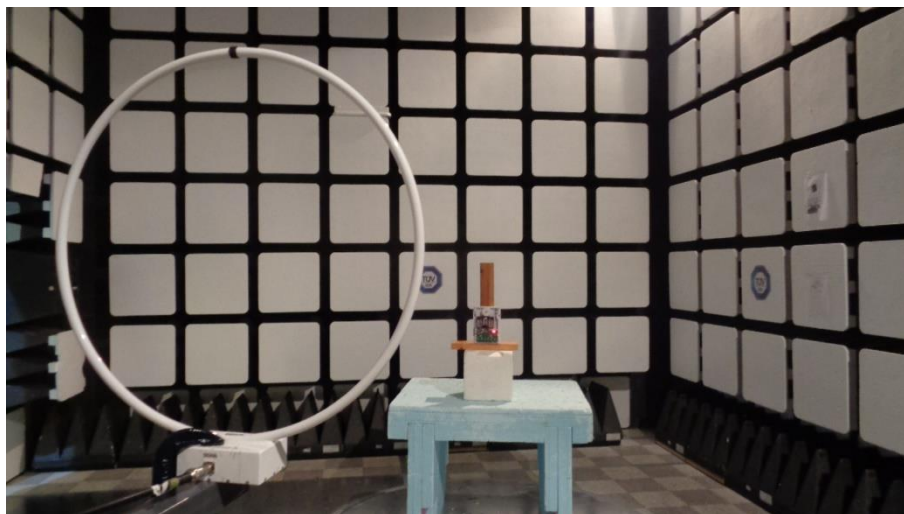
Photo 10: Setup – Tx Unwanted Emissions – SR250 – 25MHz to 30MHz
