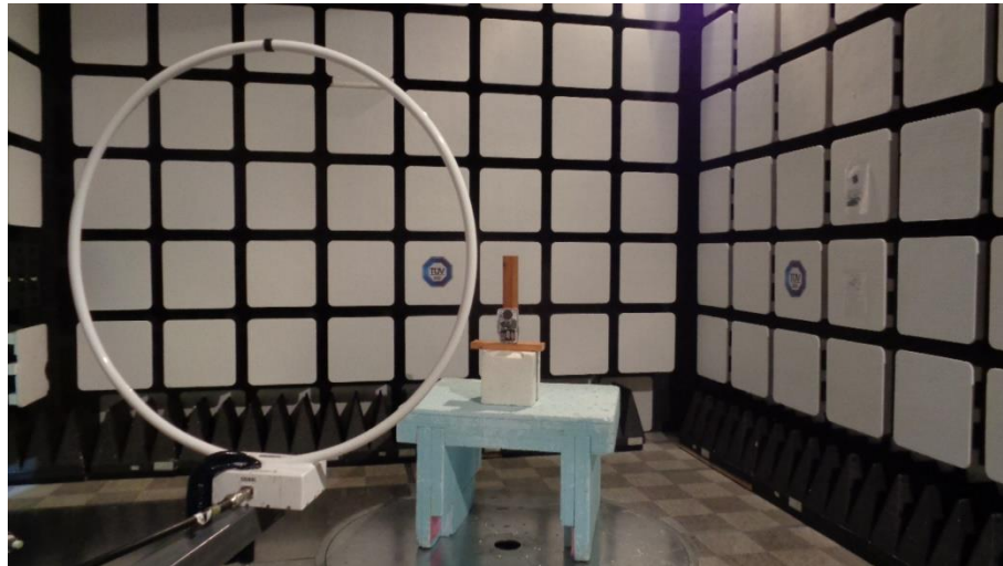
Photo 10: Setup – Tx Unwanted Emissions – SR230 – 25MHz to 30MHz
