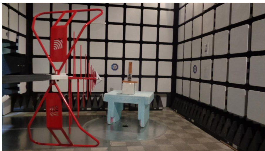
Photo 12: Setup – Tx Unwanted Emissions – SR230 – 30MHz to 1GHz – Vertical Polarization
