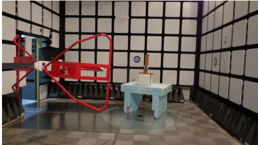
Photo 11: Setup – Tx Unwanted Emissions – SR230 – 30MHz to 1GHz – Horizontal Polarization
