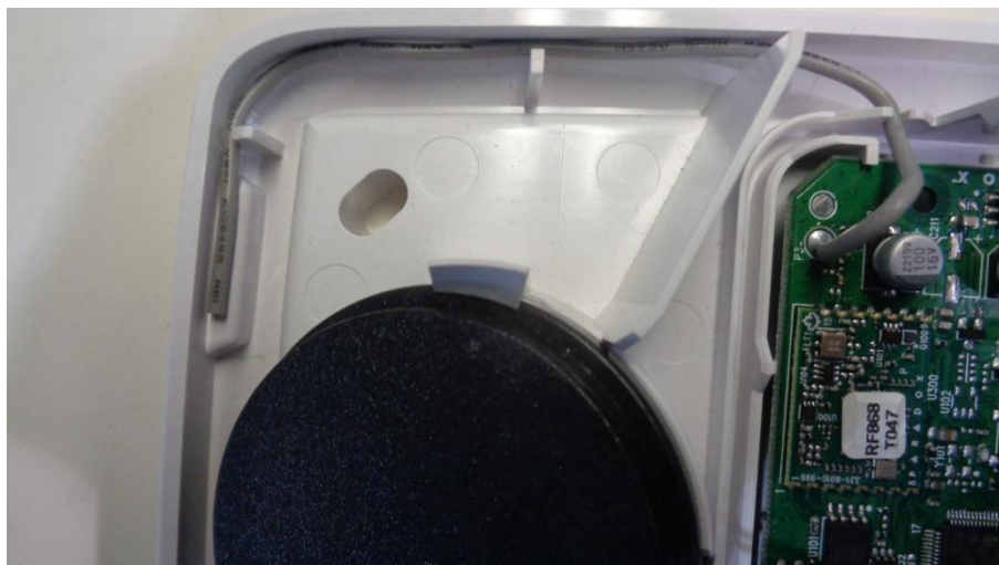
Photo 7: EUT – SR230– Antenna – Grey Cable
