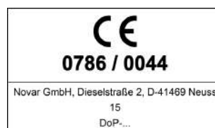
Fig. 4: CE marking in accordance with the Construction Products Regulation (CPR)
