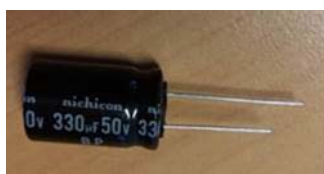
Fig. 20: Sounder End of Line Capacitor
